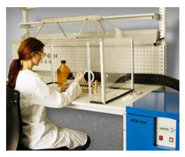
Image 6: Half-open system as capturing element - connected to a fume extraction system via a hose
