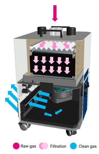
When this procedure is used, the filter is filled with a mixture of activated carbon and chemisorption medium or the activated carbon is replaced in its entirety by the chemisorption medium.
