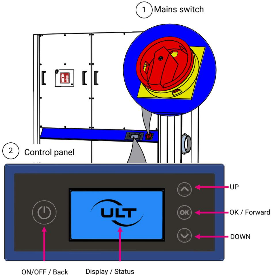
The control of the unit and the indication of the current unit status are performed via the display and the buttons of the control panel.
