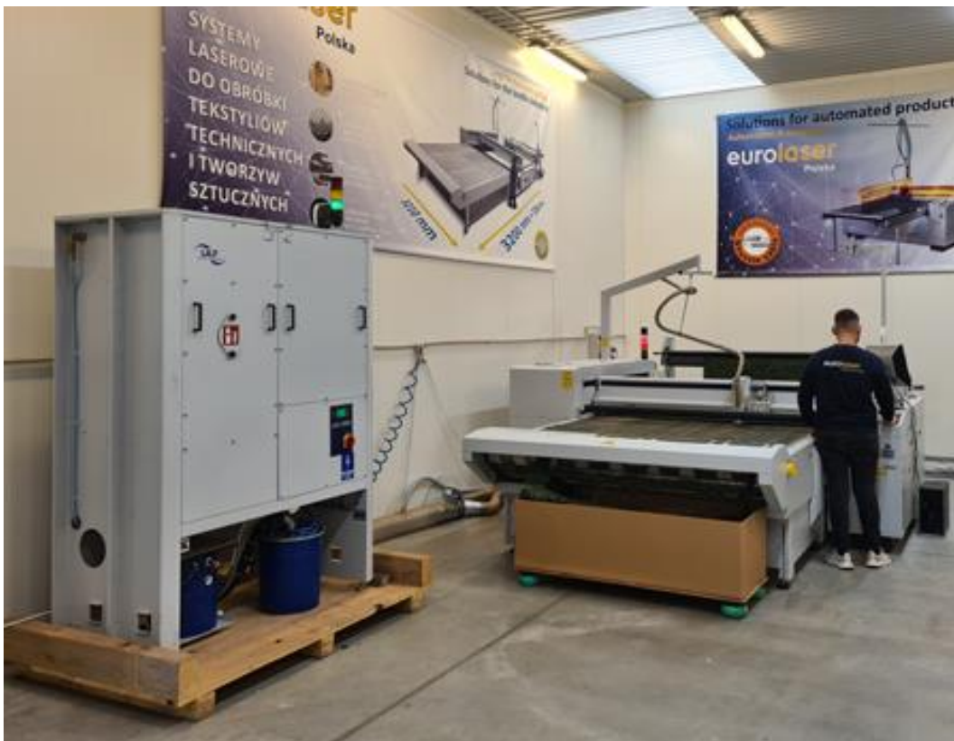
Image 3: The LAS 800 laser fume extractor (left) purifies air from laser fume and dust
