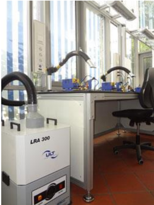
Image 4: Training area for hand soldering seminars in the SEHO Academy with extraction installations at each workplace
